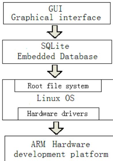
**Fig. (3).** The master control platform architecture of ARM noise data control module.
