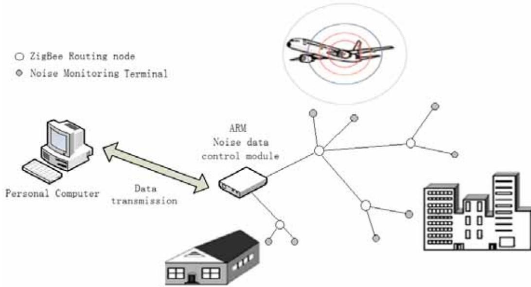
Fig. (1). The airport noise data collection system based on wireless sensor networks.
