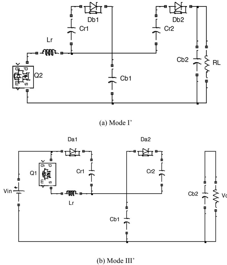
Fig. (4). Corresponding topologies for the sneaking operational modes
