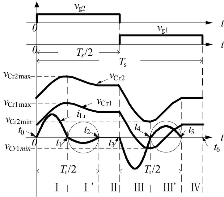
Fig. (5). Waveforms of the RSC converter with sneaking operational modes. ( $f_r > 2f_s$ ).
