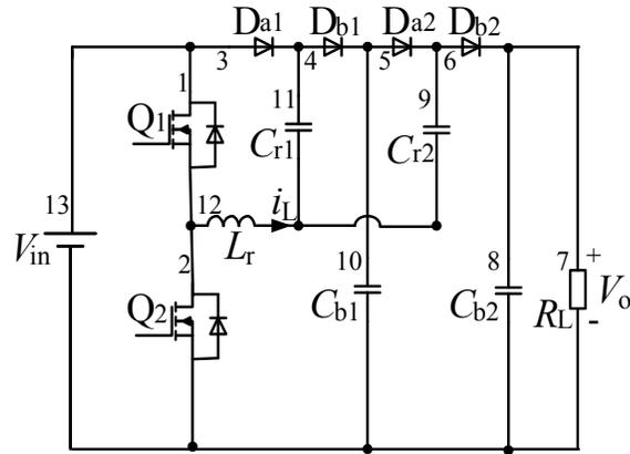
Fig. (1). A three-stage step-up RSC converter.
