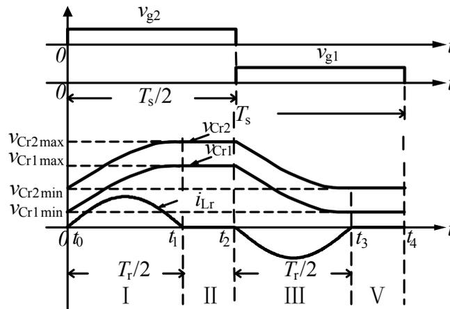
Fig. (2). Waveforms of  $i_{Lr}$  and  $v_{Cr}$  of the RSC converter.
