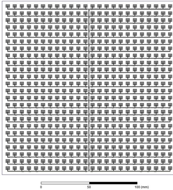
**Fig. (1).** Layout of 24×24 microstrip array.
