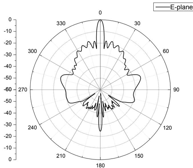
**Fig. (8).** E-plane simulation radiation pattern of microstrip array.
