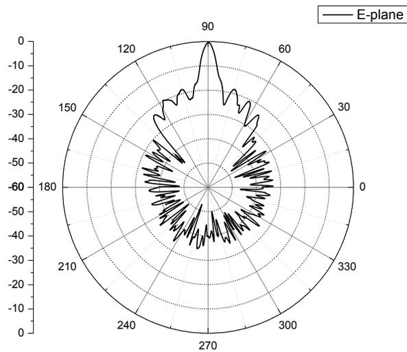
Fig. (11). E-plane radiation pattern of measure.
