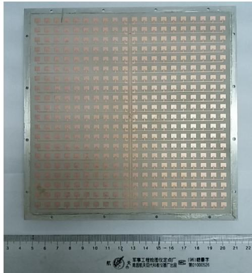
Fig. (9). Photo of microstrip array antenna.
