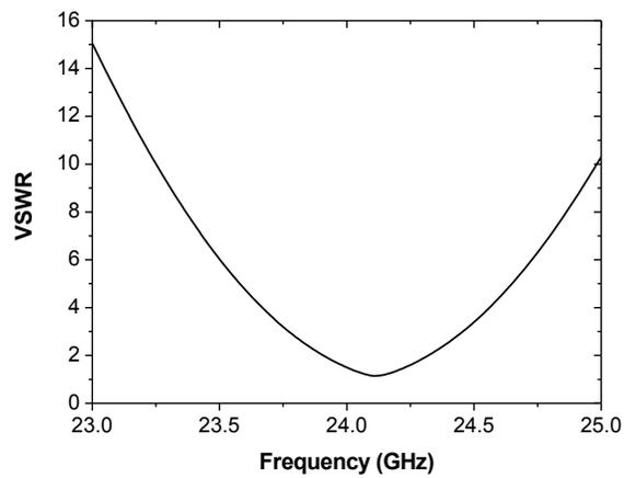
**Fig. (3).** VSWR diagram of microstrip unit.
