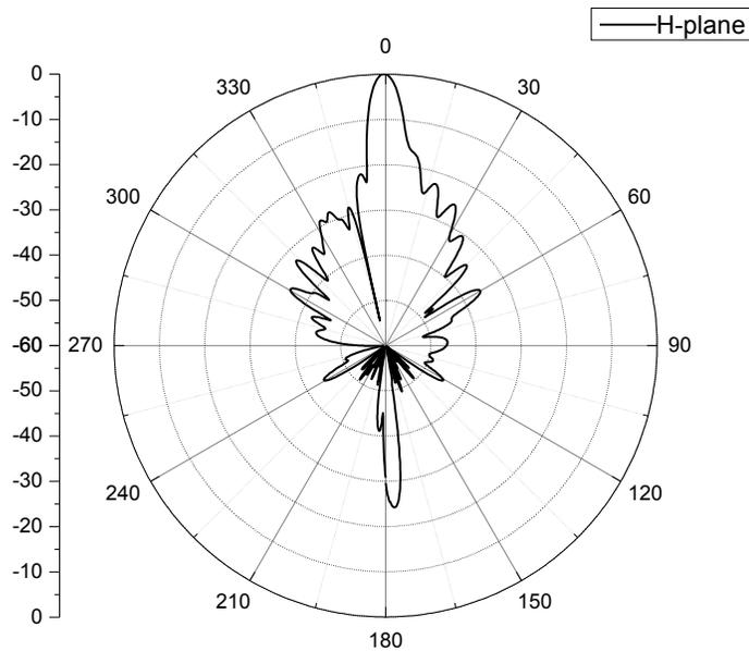
**Fig. (7).** H-plane simulation radiation pattern of microstrip array.
