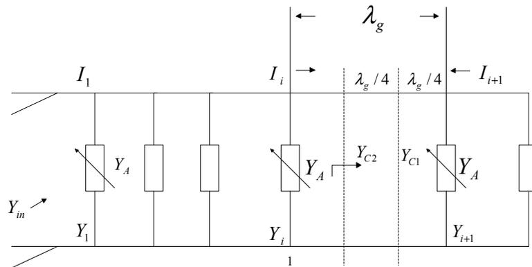
Fig. (6). Equivalent circuit model of feeding network.
