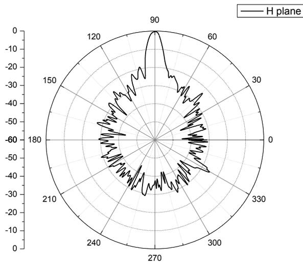
Fig. (10). H-plane radiation pattern of measure.
