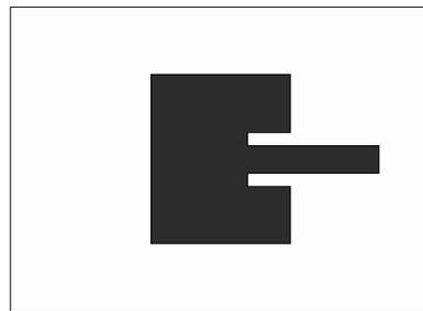
**Fig. (2).** Structure of microstrip resonator unit.
