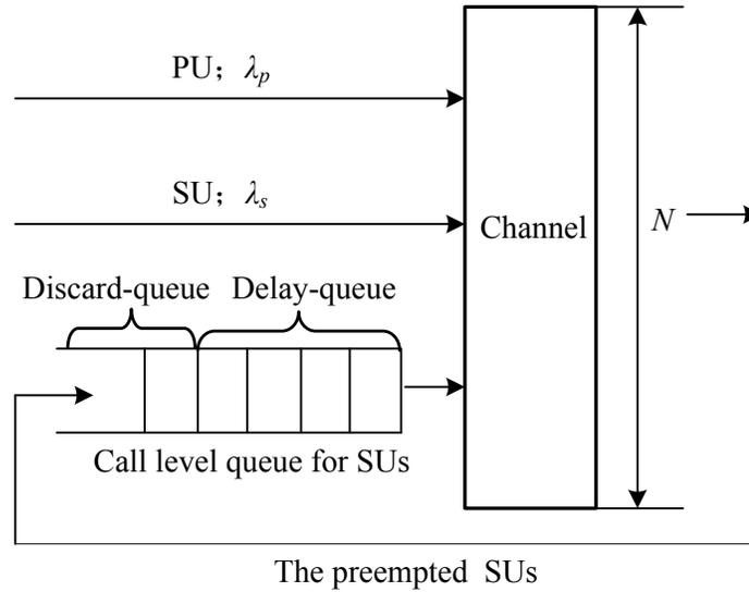
**Fig. (1).** Call level model for a CRN.
