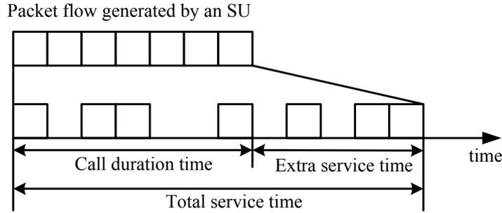
Fig. (2). Packet level model for a CRN.
