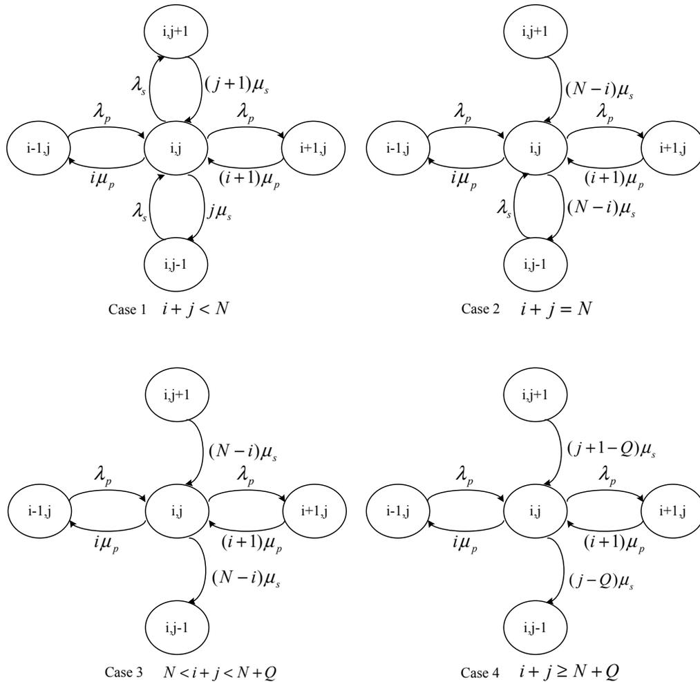
Fig. (3). State transition diagram of a CRN.
