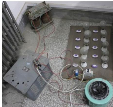
Fig. (9). APF prototype and nonlinear load.
