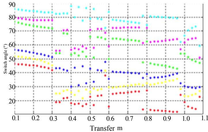
Fig. (5). Five level MSHE-PWM Solution Trajectory When  $k/m=3/3$ .
