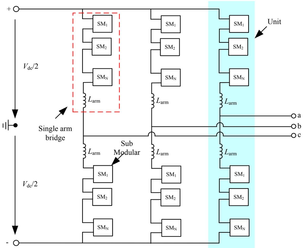
Fig. (1). MMC Topology Structure.
