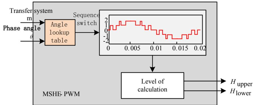
Fig. (3). MMC Topology MSHE - PWM Principle.
