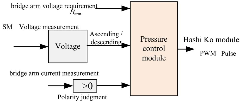
Fig. (2). Voltage Balance Principle of SMs.
