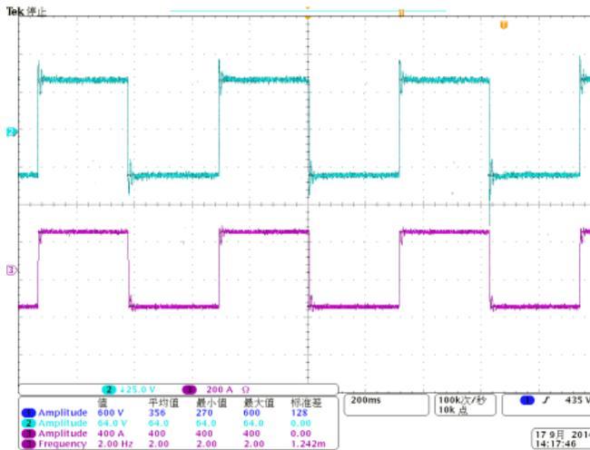
Fig. (14). Output voltage and current waveforms of transmitter transmitting electrode with single loop.
