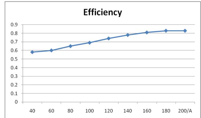
Fig. (16). Measure efficiency of marine electromagnetic detection transmitter.
