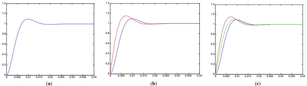
Fig. (4). System response with different zeros.
