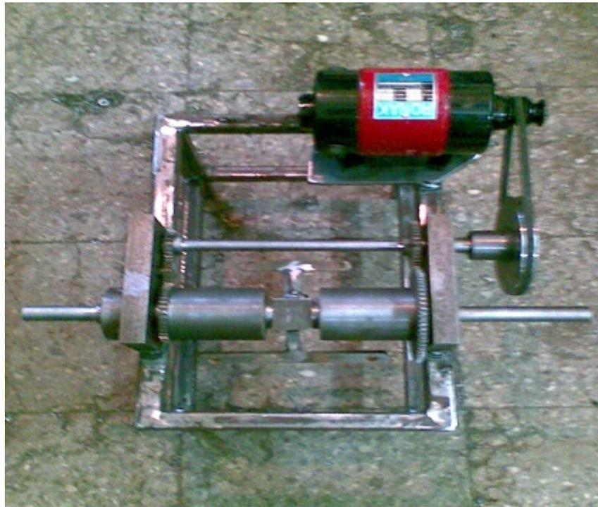
**Fig. (4).** Fabricated assembly of mechanical power amplifier.
