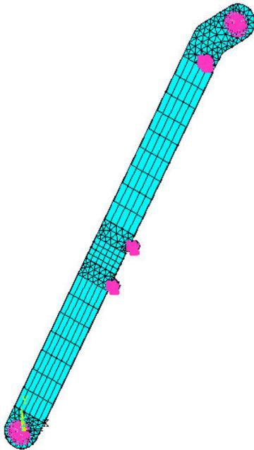
Fig. (7). Finite element model of the first arm of the boom system.
