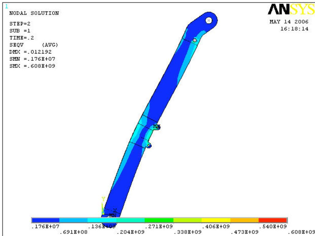
Fig. (10). The equivalent stress distribution of the first arm in ANSYS.
