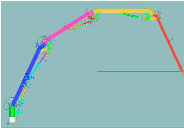
Fig. (5). Kinematics simulation in ADAMS.
