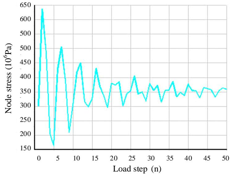
Fig. (9). The time-history curve of stress for a node on the flexible arm.
