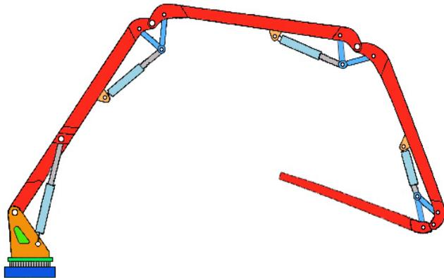
**Fig. (3).** A four-section boom system.
