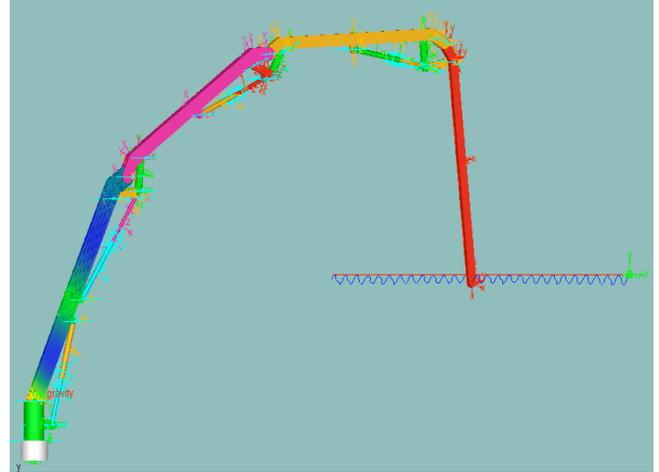
Fig. (8). Kinematics simulation of the boom system with the flexible arm (the first arm) in ADAMS.
