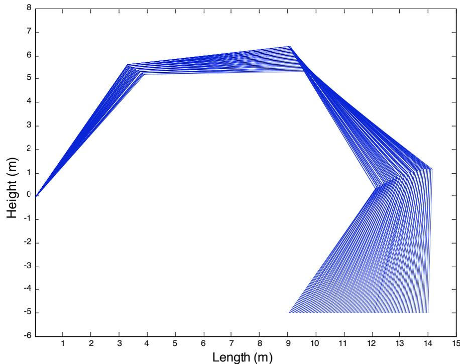
**Fig. (4).** The movement postures of the boom system for a straight-line trajectory.
