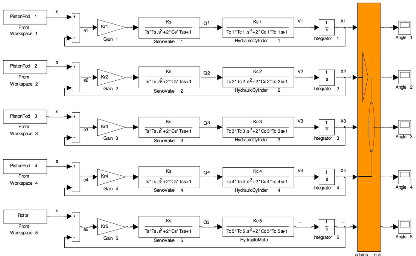
Fig. (6). The control scheme of Co-simulations in ADAMS and Matlab/Simulink.
