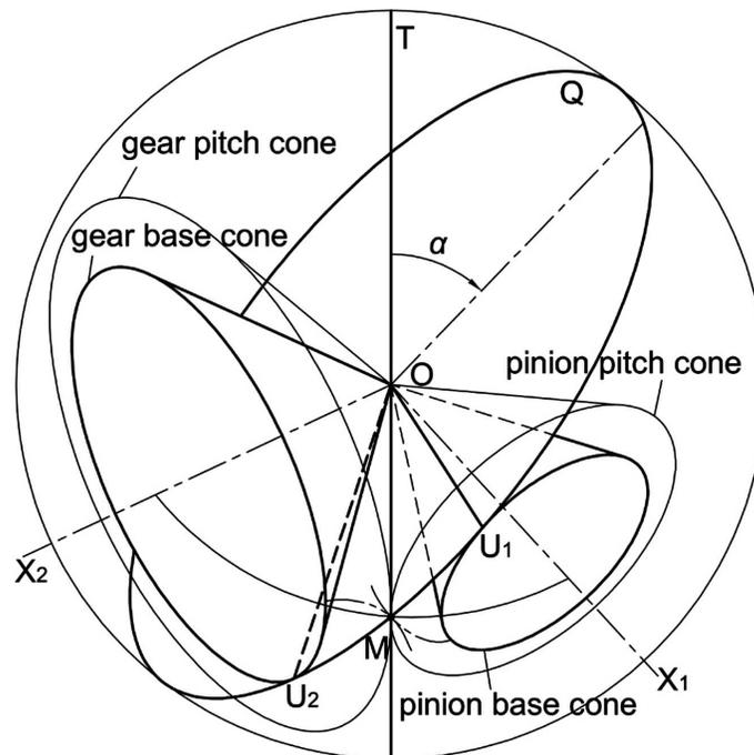
Fig. (2). Schematic of a bevel gear drive.
