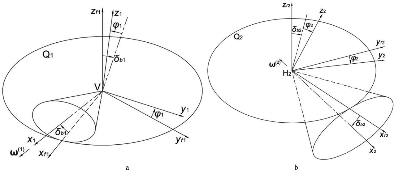
Fig. (8). Coordinate systems  $S_1, S_2$ .
