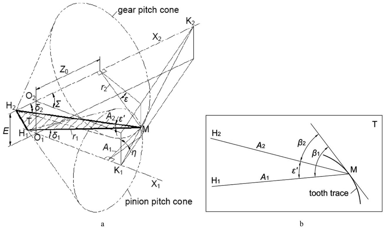
Fig. (1). Basic geometry of hypoid gears.
