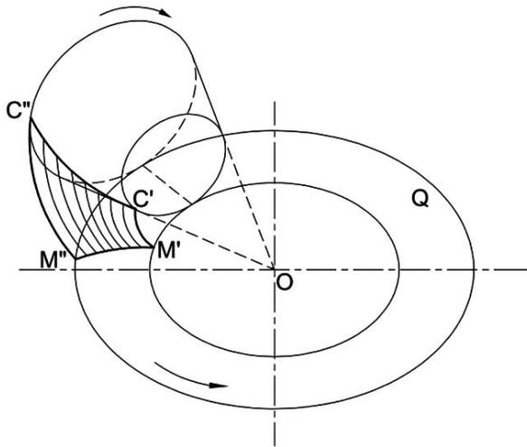
Fig. (3). Principle of generating-line method.
