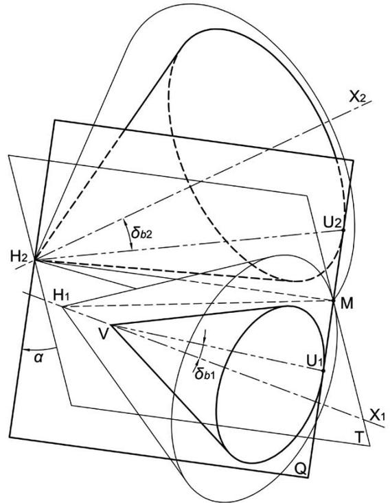
Fig. (4). Geometry of cutting hypoid gears.
