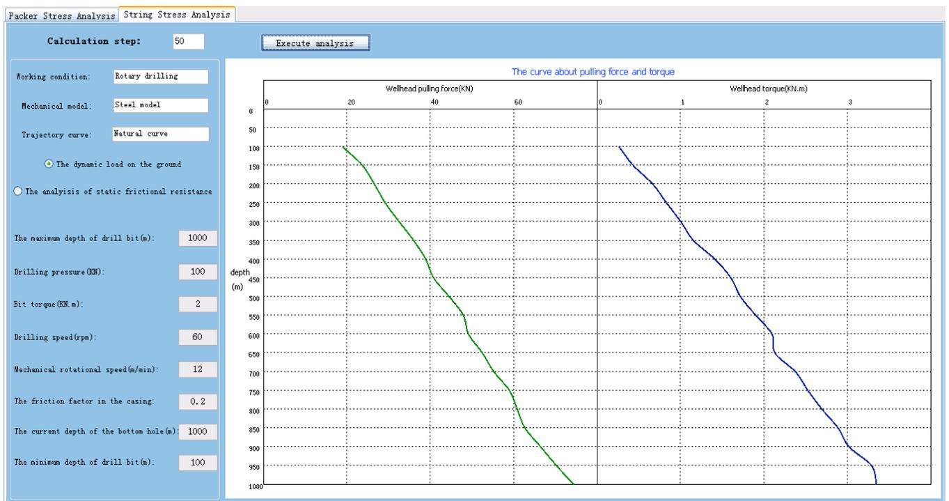
Fig. (4). Dynamic frictional resistance analysis.
