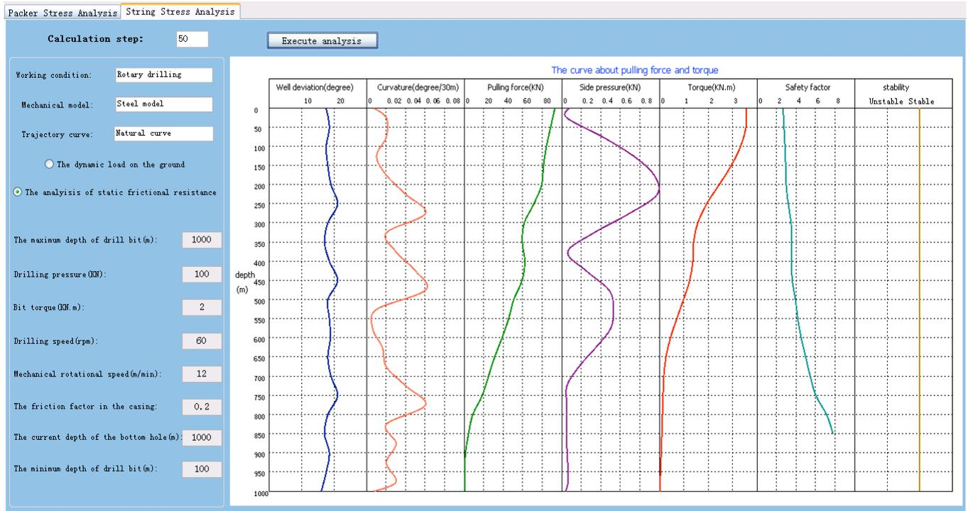
Fig. (3). Static frictional resistance analysis.
