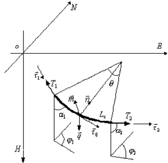
Fig. (2). The tubular column unit in the three-dimensional wellbore.
