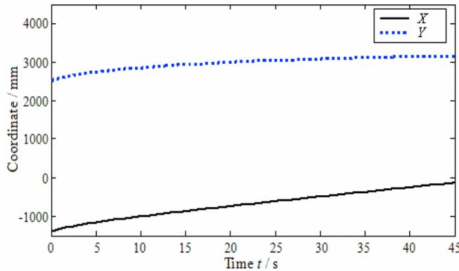
**Fig. (11).** Position curve of the center of gravity of garbage container.
