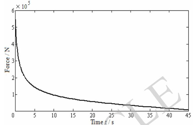
**Fig. (13).** Force curve of the lifting cylinder.
