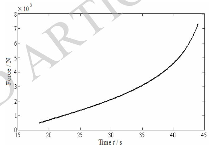
**Fig. (9).** Force curve of the lifting cylinder in the second stage.
