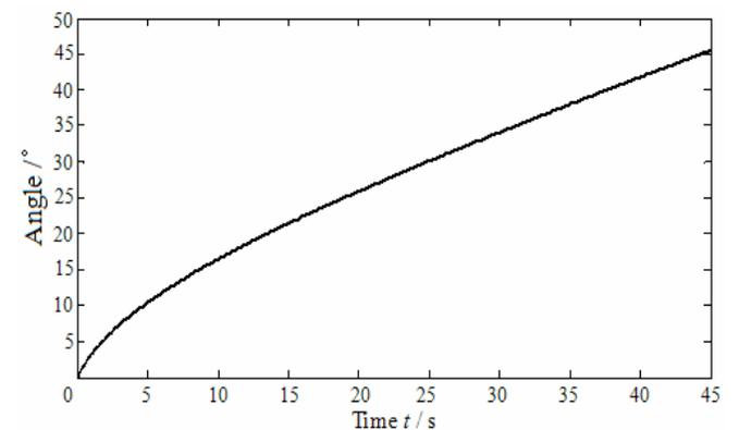
**Fig. (10).** Variation curve of dumping angle.
