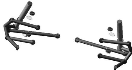
Fig. (3). The model of rear suspension.
