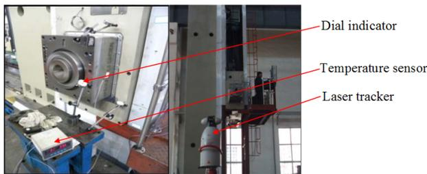
Fig. (8). The measuring system of field experiment.
