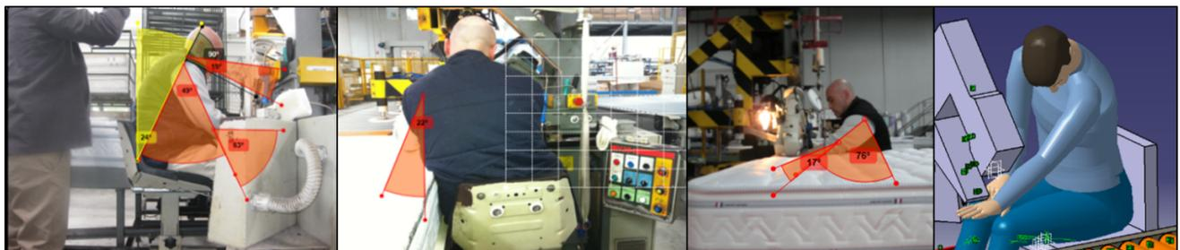
Fig. (6). Angles' detection: sewing.
