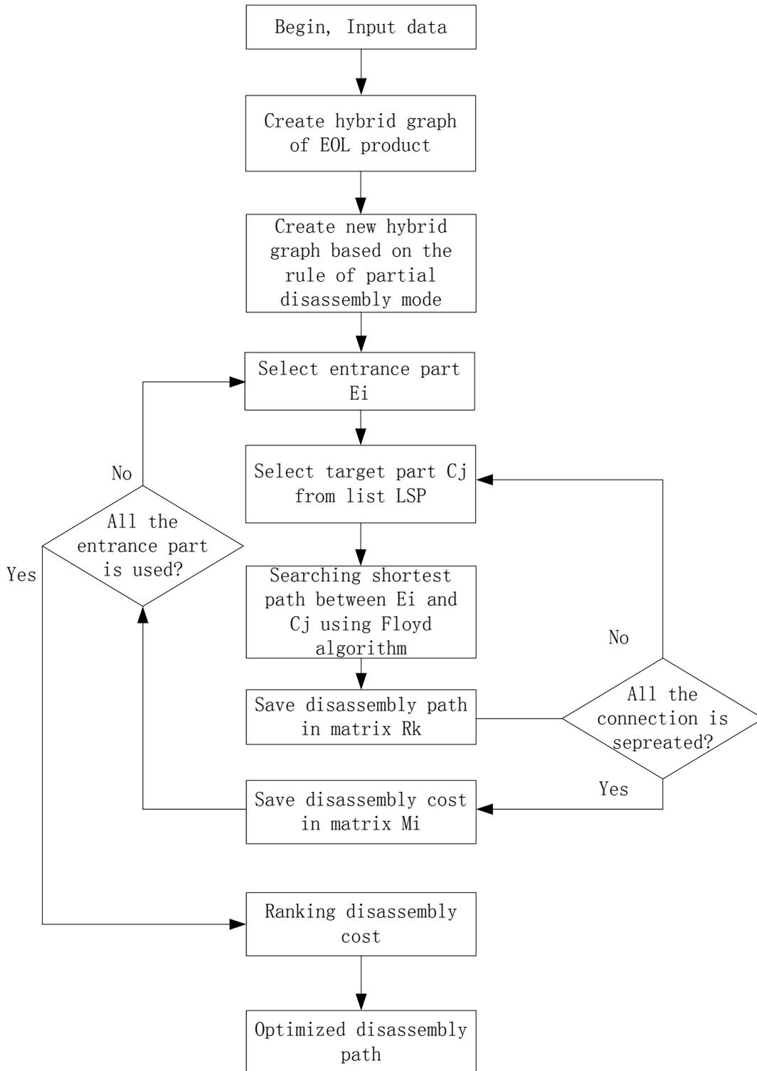
Fig. (6). Algorithm for searching optimized disassembly sequence.
