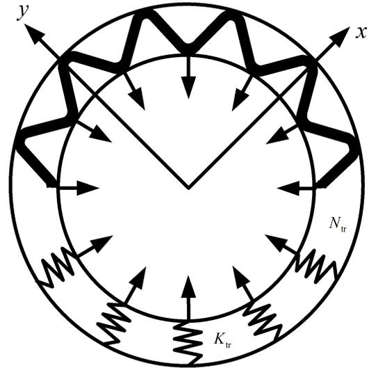
Fig. (5). Support model of tolerance ring.
