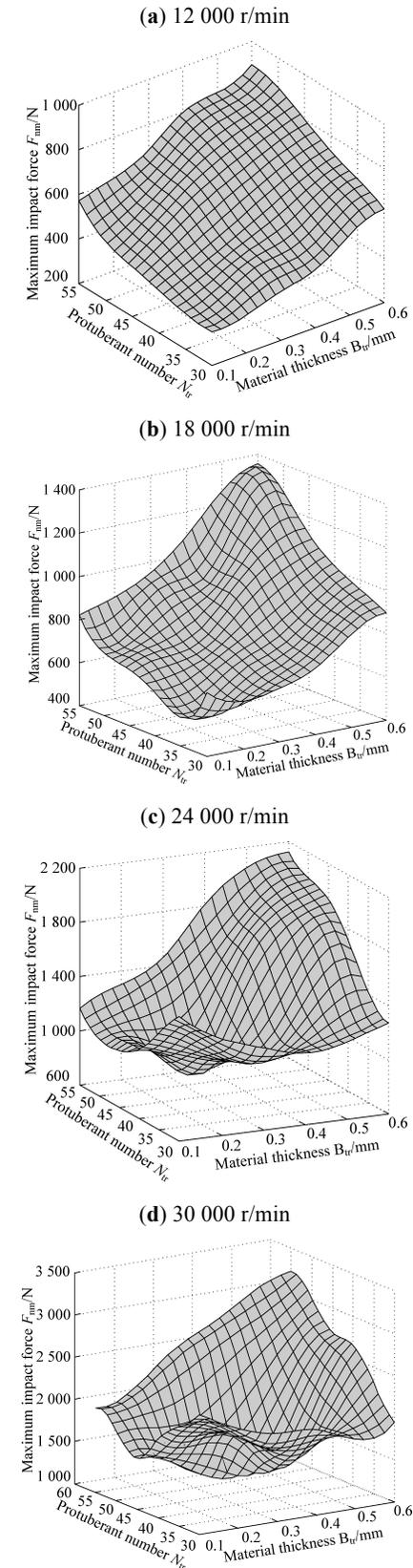
Fig. (6). Influences of tolerance ring parameters on maximum impact forces.
