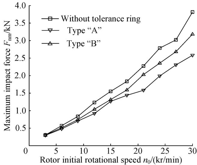
Fig. (10). Maximum impact force obtained by experiments.
