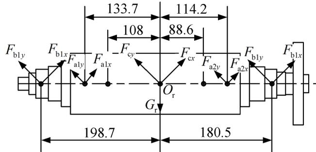
Fig. (3). Rotor force model.
