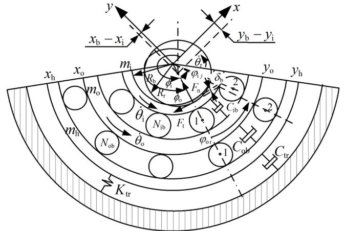
Fig. (4). Contact model after rotor drop.
