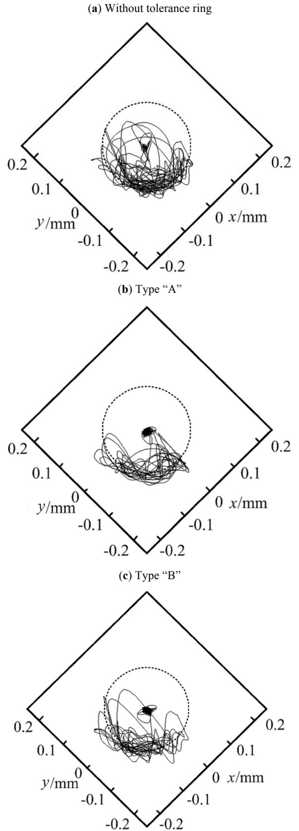
**Fig. (9).** Rotor orbits obtained by experiments.
