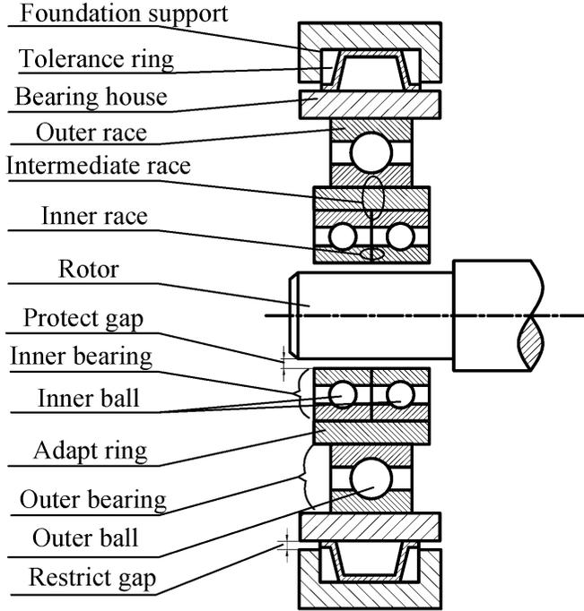
Fig. (2). Structure of analyzed DDCB.
