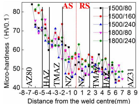
Fig. (6). Micro-hardness of different FSW parameter joints.
