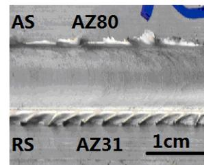
**Fig. (2).** Macrograph of friction stir welded joint.
