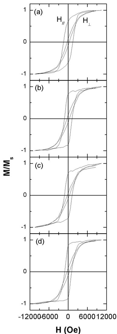
**Fig. (4).** Hysteresis loops of the  $\text{Co}_{1-x}\text{P}_x$  alloy nanowires with  $x=8.7$  wt% for different deposition time at ambient temperature: (a) 1 min; (b) 2 min; (c) 4 min; (d) 6 min.  $H_{//}$  and  $H_{\perp}$  represent that the applied field  $H$  are parallel and perpendicular to the wires axis.
