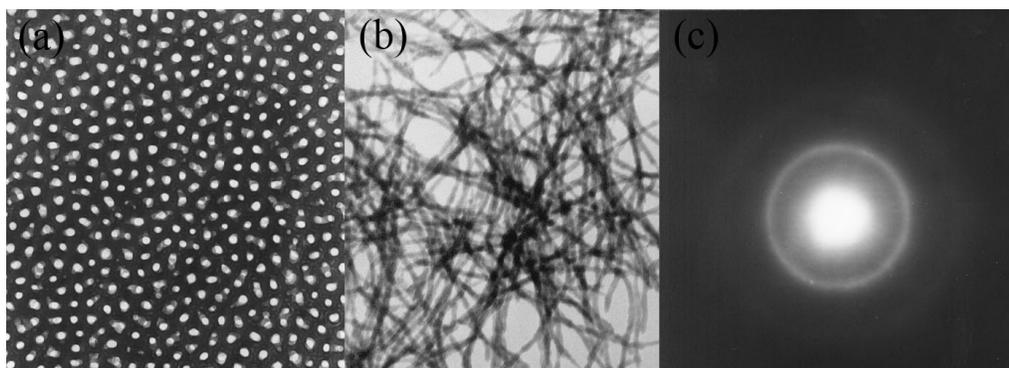
**Fig. (1).** The representative images: (a) SEM image of AAO films; (b) TEM image and (c) SAED of the  $\text{Co}_{1-x}\text{P}_x$  alloy nanowires with  $x=6.8$  wt%.
