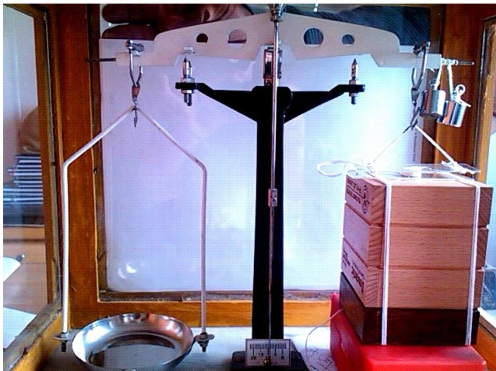
Fig. (1). Tablet mucoadhesive strength testing apparatus.
