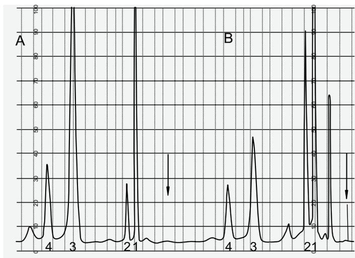
**Fig. (5).** HPLC analysis of aliquots of OHCP incubated in rat serum (pH7, 37°C) for 10 min (A) or 90 min (B). Proteinprecipitation and reaction of the aldehydes with 2,4 dinitrophenylhydrazine. 1: 2,4 dinitrophenylhydrazine, 2,3,4: dinitrophenylhydrazones of hydroxypropanal (2), aldophosphamide (3) and acrolein (4). Arrows indicate start of HPLC run.
