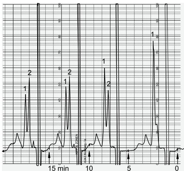
**Fig. 2a.** HPLC protocol of the formation of ALDO (2) from OHCP (1) in 0.07M phosphate buffer (pH7, 37°C), arrows indicate start of HPLC run.
