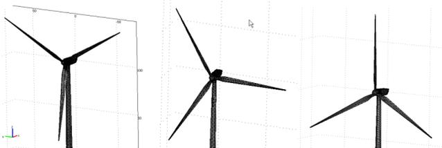
Fig. (6). Rotor orientations for the numerical simulations on lightning attachment points for the V164-7MW turbine.
