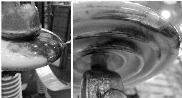
**Fig. (12).** Influence of long tail lightning current on surface of suspension insulator.
