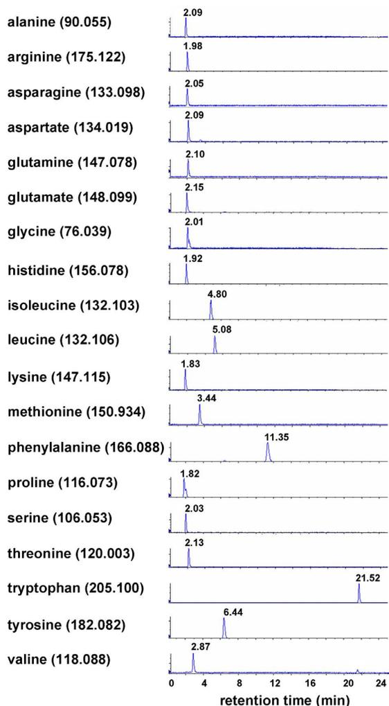
**Fig. (1).** Selective ion chromatograms for standard solution of low molecular weight compounds (LMCs) in positive electro spray ionization mode.
