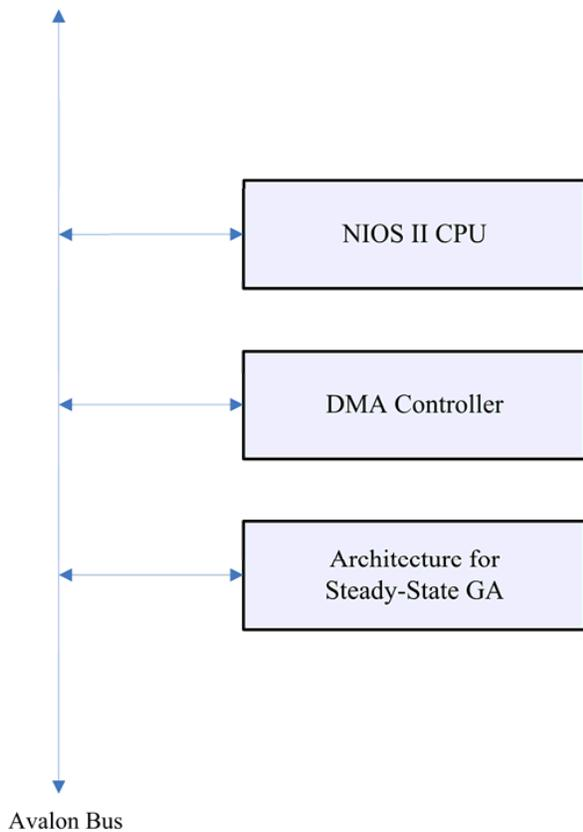
Fig. (5). The architecture of each island of the proposed distributed GA architecture.
