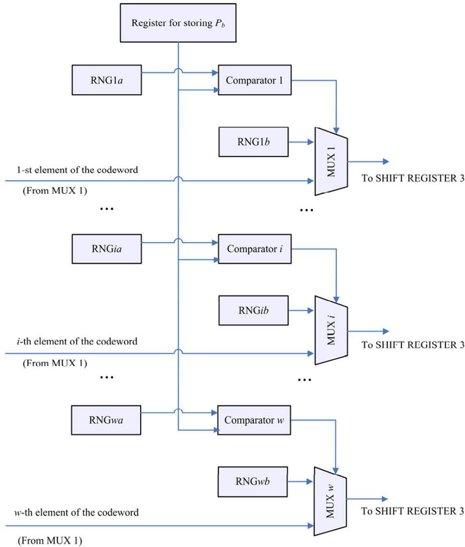
**Fig. (3).** The architecture of mutation unit.
