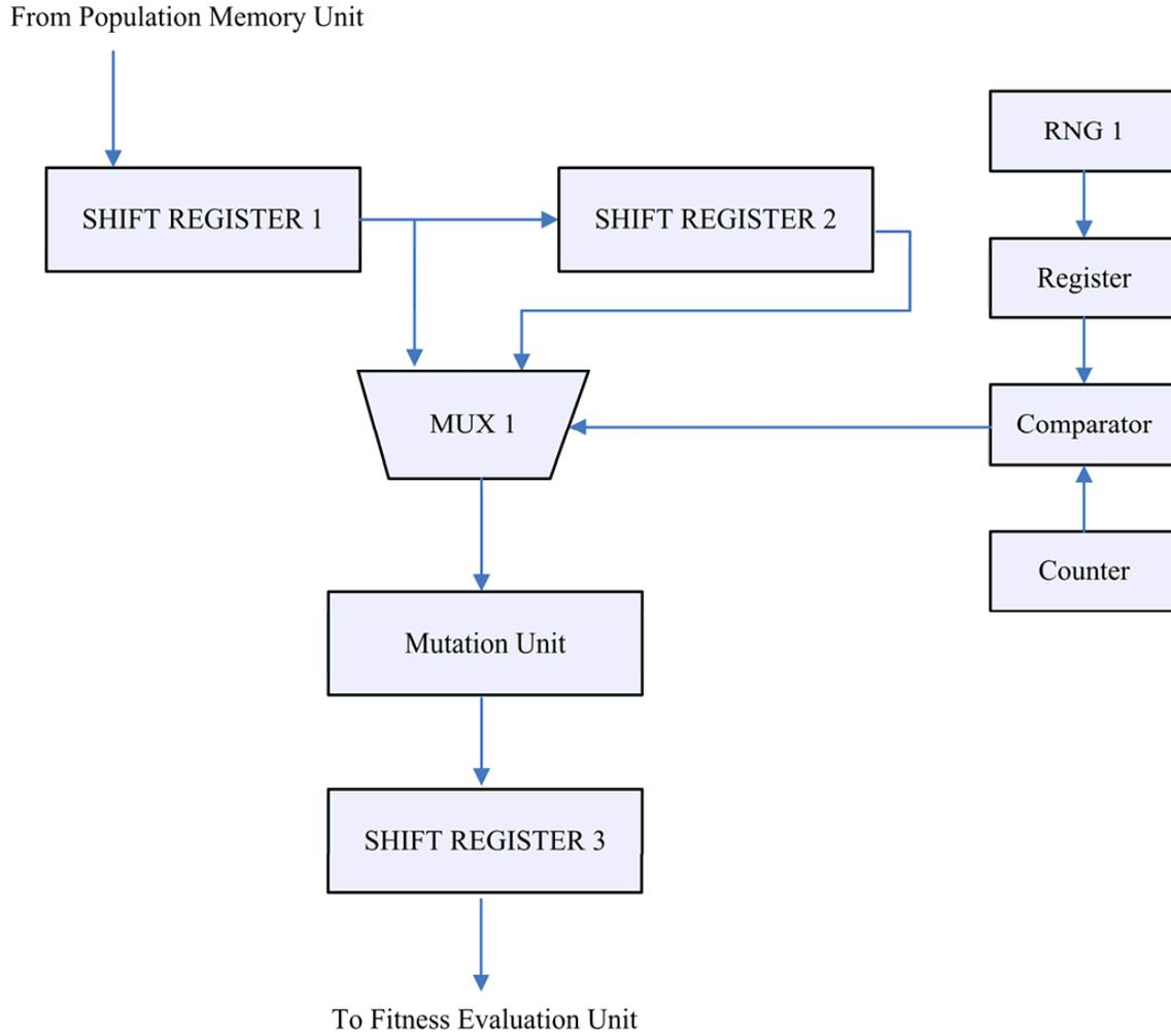
Fig. (2). The architecture of crossover and mutation unit.
