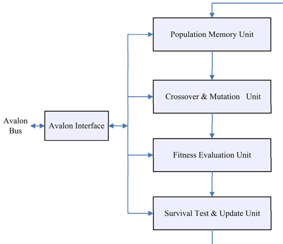
Fig. (1). The proposed hardware architecture of steady-state GA.
