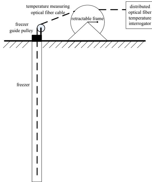
Fig. (1). Components of the detection system.
