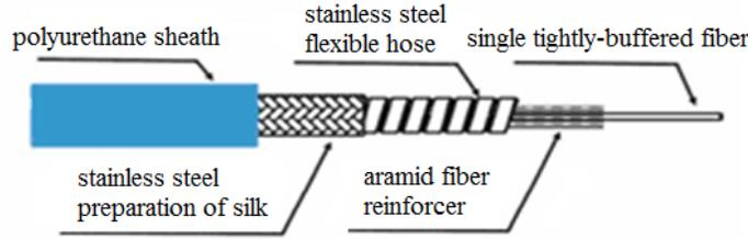
Fig. (3). The armored cable structure.
