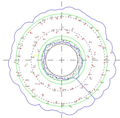
Fig. (8). The circular diagram of the frozen wall at a depth of -560m.
