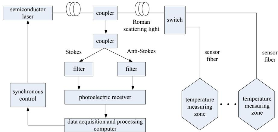
Fig. (2). Structure of the distributed optical fiber temperature interrogator.
