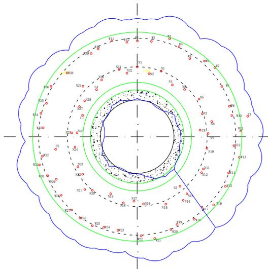
Fig. (7). The circular diagram of the frozen wall at a depth of -490m.
