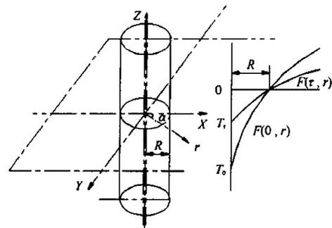
Fig. (4). The mathematical model of temperature rise in single span frozen column.
