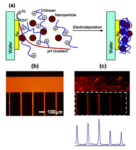
Fig. (7). Electrodeposition of Chitosan can mediate nanoparticle assembly. (a) Mechanism of chitosan-mediated nanoparticle deposited on the cathode. (b) Photomicrograph of silicon wafer patterned with 20  $\mu$ m gold lines for deposition. (c) Fluorescence photomicrograph showing spatially localized deposition of 100 nm fluorescent latex spheres from a 1% chitosan solution at pH = 5. [98].
