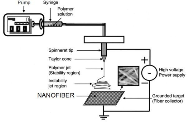
Fig. (4). Schem of electrospinning system.
