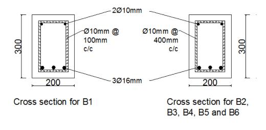
Fig (2). Cross section of specimens.
