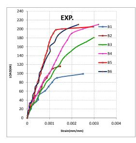
Fig. (8). Load-compression strain of all specimens.
