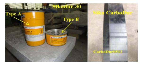
Fig (3). Manufactured forms of CFRP materials.
