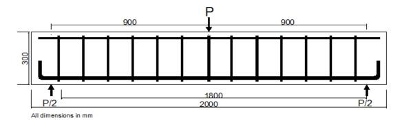
Fig. (1). Specimens details of B1.
