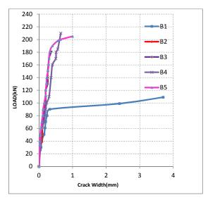
Fig. (7). Load-crack width of all specimens.
