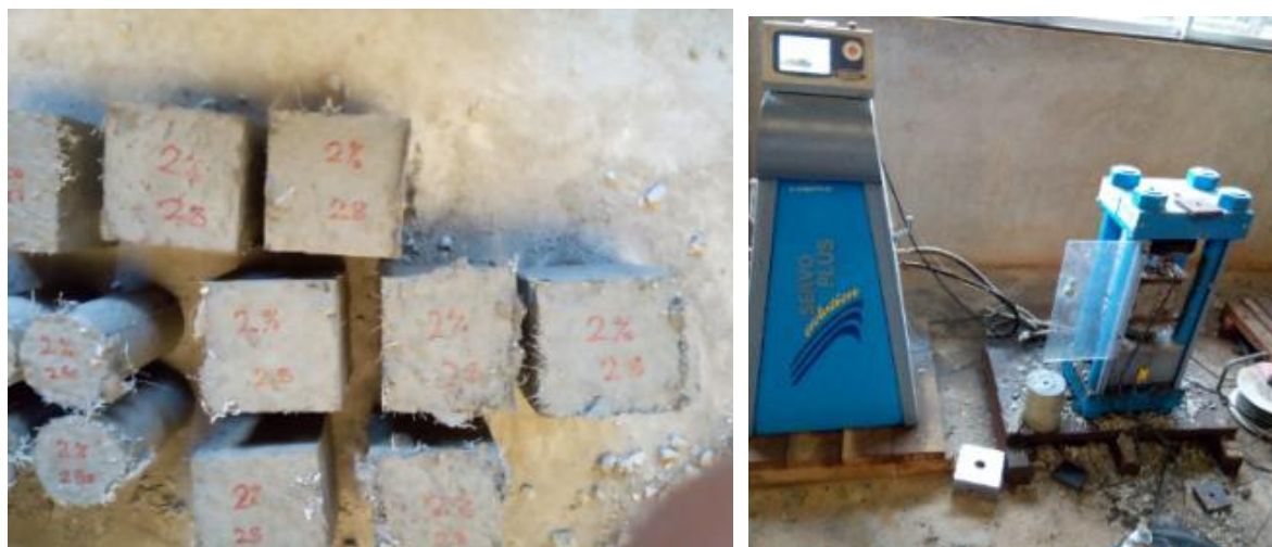
Fig. (2). (a) Test Samples ( M_{2.0} ) (b) Servo-Plus Evolution UTM
