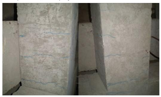
Fig. (9). Crack development of No.2 specimen in the cyclic load.
