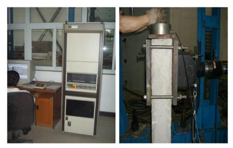
Fig. (4). MTS system and data collection system.
