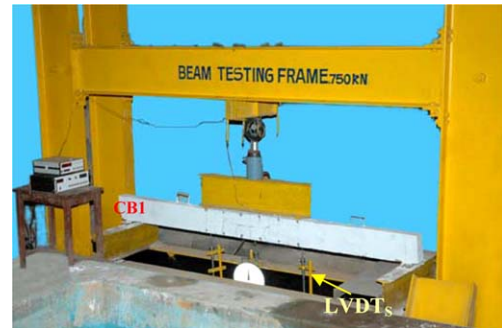
Fig. (4). Test Set Up for Static Loading.
