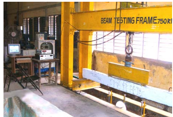
Fig. (5). Test Set Up for Compression Cyclic Loading.
