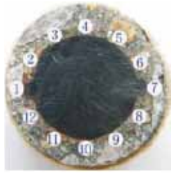
Fig. (2). Measured point label for microscopic test.
