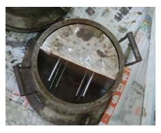
Fig. (3). Sketch of wooden model in steel mould.
