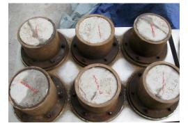
b. without slurry (0.2MPa) **Fig. (4).** Seepage state of the flat joints.
