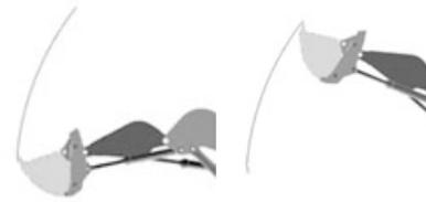
Fig. (12). The trajectory of the bucket tip in the boom lifting process.
