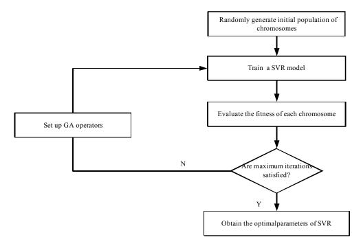
Fig. (1). The operational process of genetic support vector regression algorithm.
