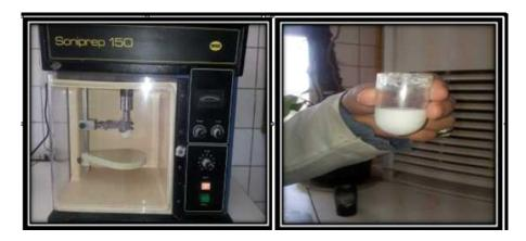
Fig. (3). TiO2 Nanofillers were well dispersed in the monomer by a probe sonication apparatus.
