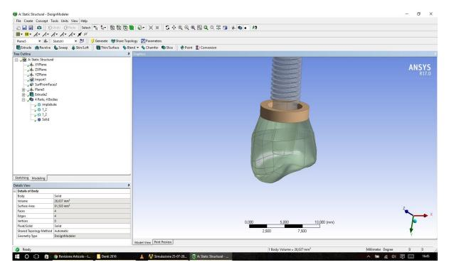
Fig. (1). Creating a three-dimensional model of the dental implant with a single crown.
