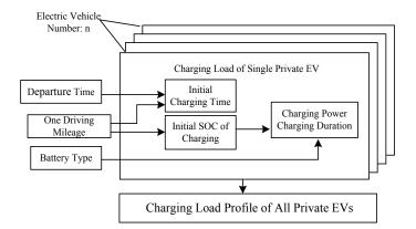
Fig. (3). Diagram of EVs charging load calculation.
