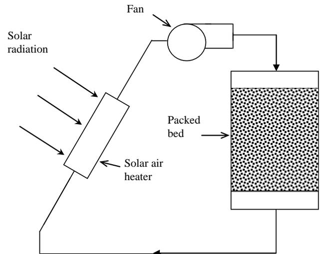
Fig. (1). Schematic of packed bed solar energy storage system.
