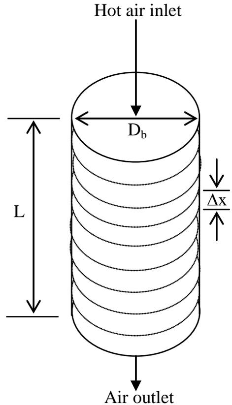
**Fig. (2a).** Packed bed (voids are not shown).
