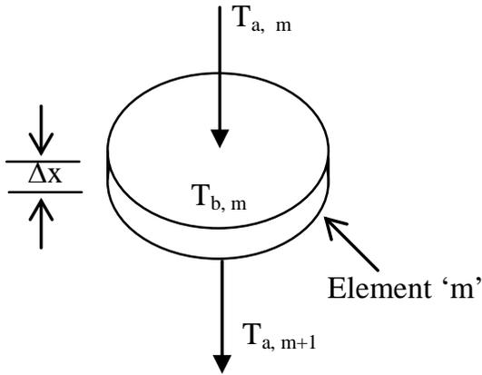
Fig. (2b). Element ‘m’ of packed bed.
