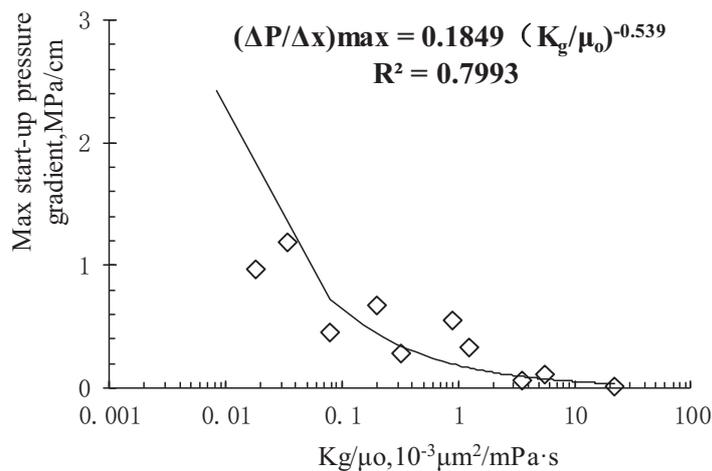
Fig. (7). Relationship between maximum start-up pressure gradient and  $kg/\mu_o$ .
