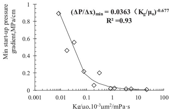
Fig. (5). Relationship between minimum start-up pressure gradient and  $k_g/\mu_o$ .
