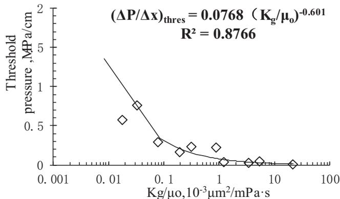
Fig. (6). Relationship between threshold pressure and  $k_g/\mu_o$ .
