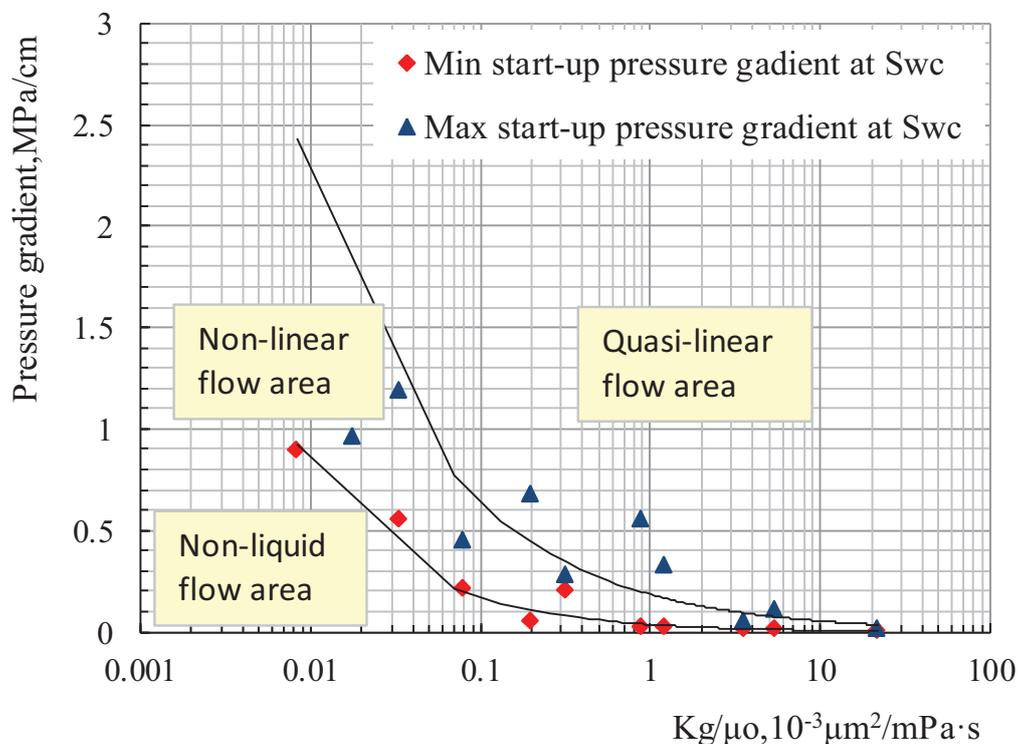
Fig. (8). Diagram for determining the min and max start-up pressure gradient of super heavy oil in different permeable reservoirs.
