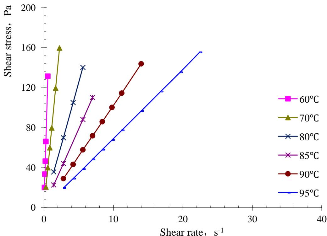
Fig. (2). Rheological curves of super heavy oil from Shengli Oilfield at different temperatures.
