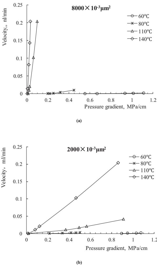
**Fig. (4).** Velocity-pressure drop curves with different permeable sand packs at different temperatures.
