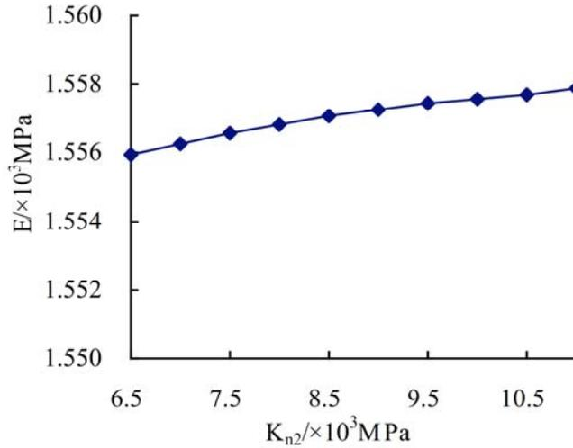
Fig. (4). The relationship between the elastic modulus  $E$  of coal body and the normal stiffness  $k_{n2}$  of face cleat.
