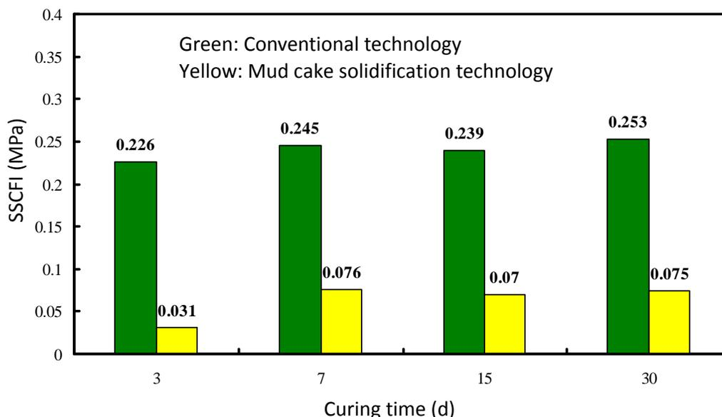
Fig. (2). Comparison of SSCFI in conventional technology and mud cake solidification technology.
