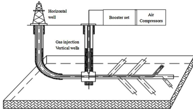
**Fig. (1).** The structure of the coalbed methane cavity aerated underbalanced drilling.
