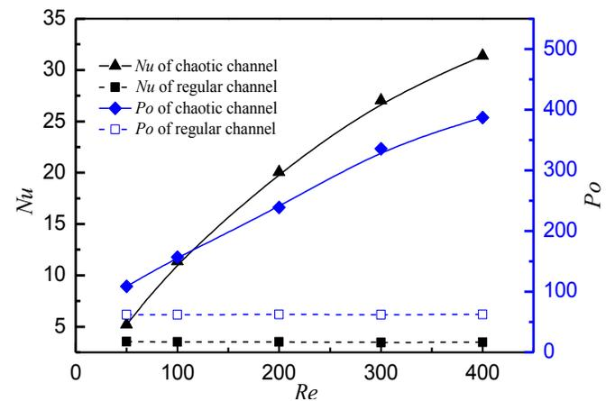
Fig. (11). The relationship between  $Nu$  number and  $Po$  &  $Re$  number in two kinds of channels.
