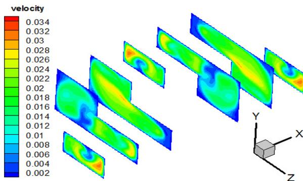
Fig. (5). Velocity distribution diagram of chaotic channel.
