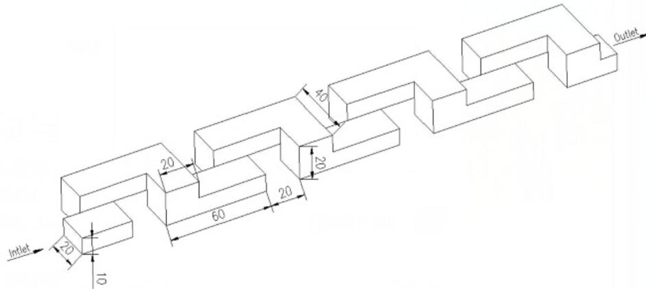
Fig. (1). Structure and size of chaotic channel.
