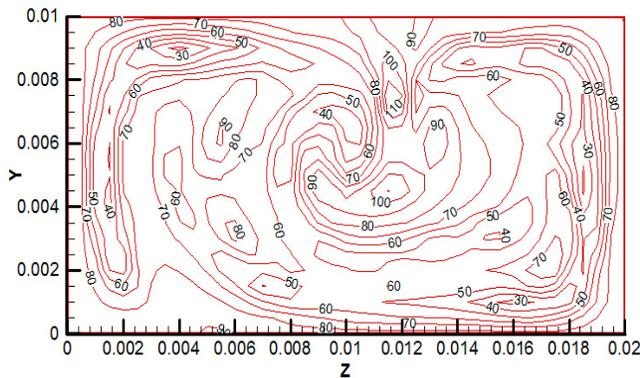
Fig. (9). Synergy angle distribution diagram of chaotic channel.
