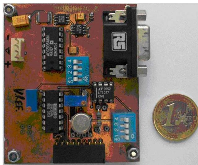
**Fig. (12).** Picture of the miniaturized electronic plate that functions as a potentiostat. (*Talanta* 75(2008)1208).
