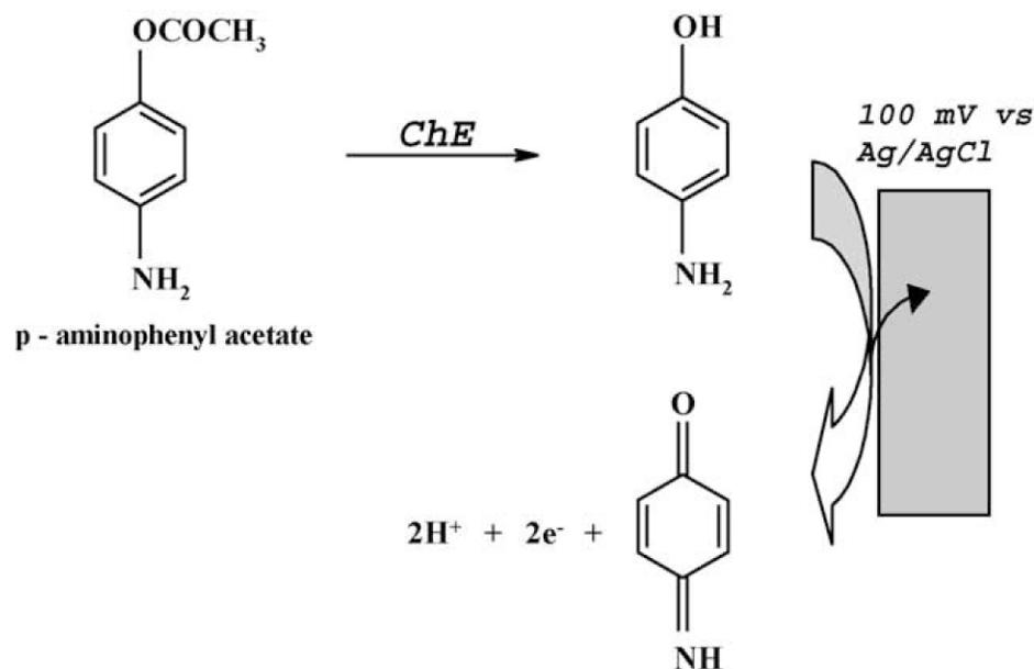
**Fig. (7).** Mono-enzymatic amperometric ChE biosensor based on p-aminophenyl acetate as substrate. (*Biomolecular Engineering*, 2006, 23, 1).
