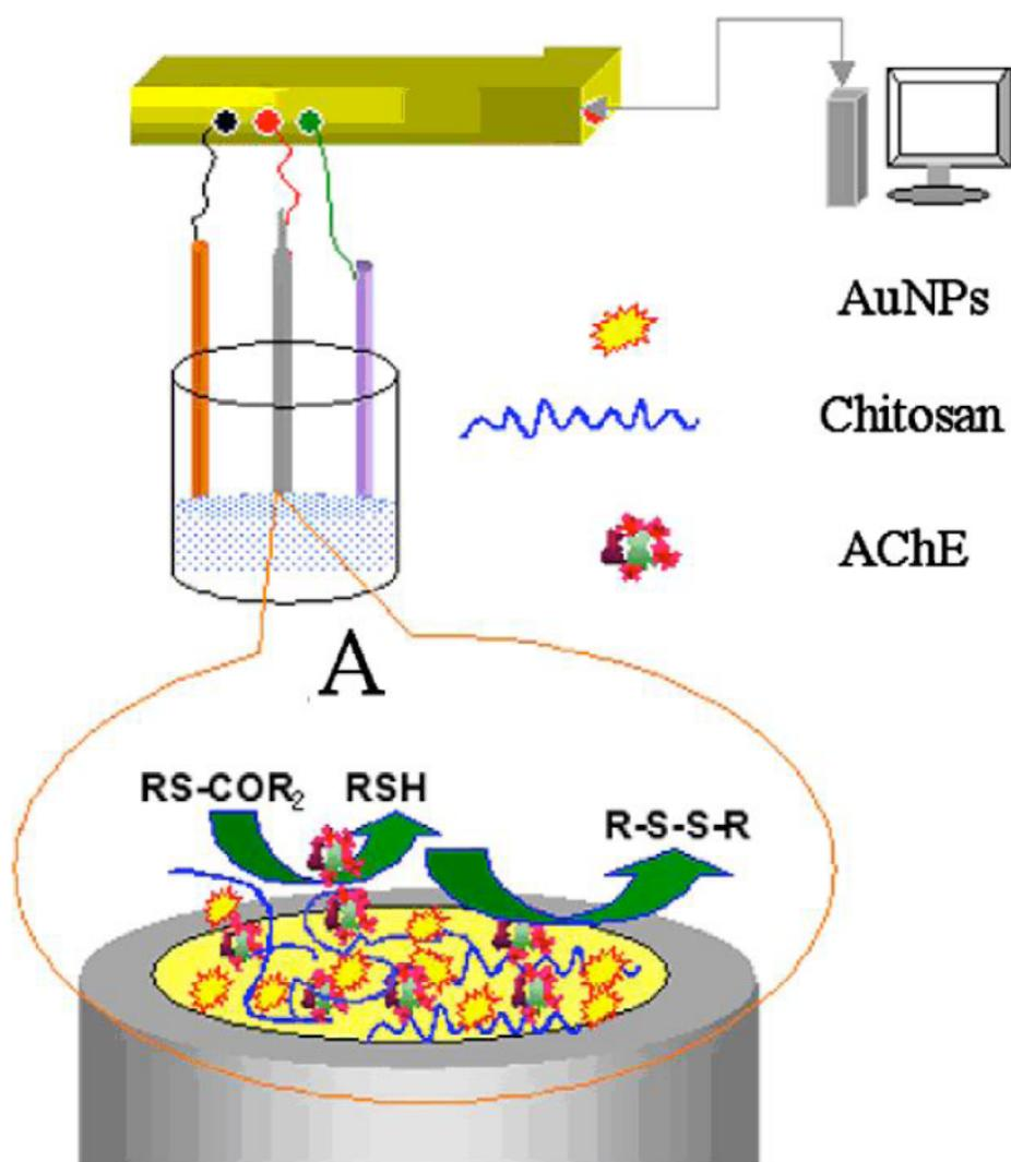
**Fig. (4).** Mechanism of constructed biosensor based on one-step electrodeposition. (A) Megascopic interface of AChE/CHIT–GNPs modified gold electrode. (*J. Electroanal. Chem.*, 2007, 605, 53).
