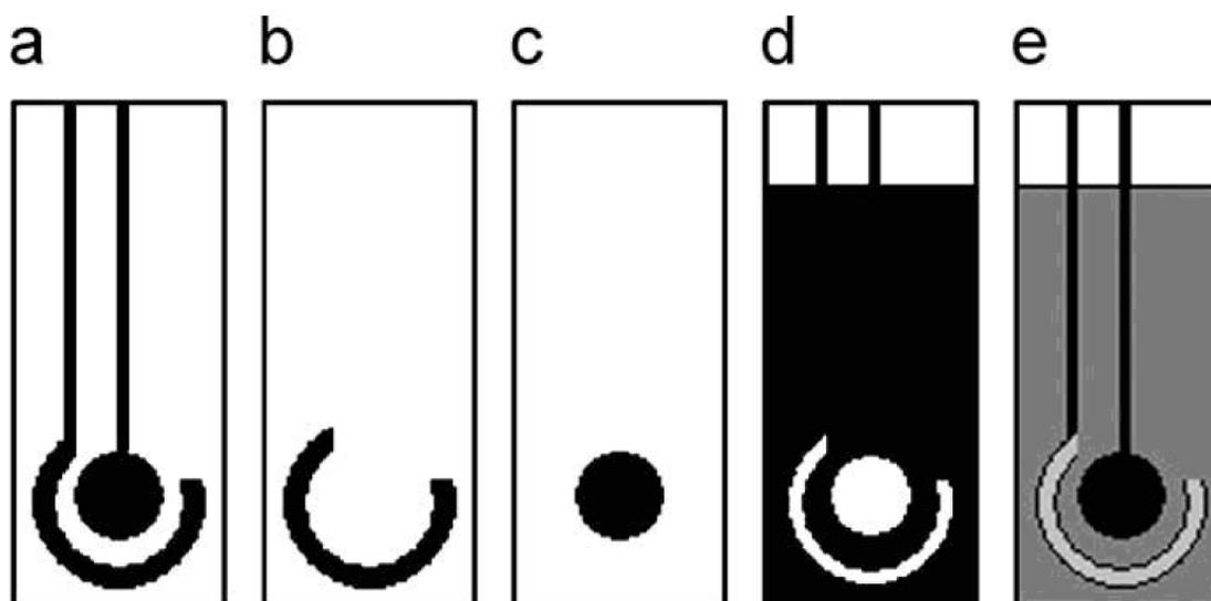
**Fig. (5).** Design of screens for 2-electrode biosensor: (a) basal track; (b) reference electrode; (c) working electrode; (d) insulation coating; (e) schematic of two-electrode screen-printed sensor. (*Ecotoxicology and Environmental Safety*, 2008, 69, 556).
