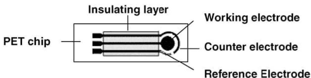
**Fig. (6).** The diagram of the integrated three screen-printed electrodes. (*Talanta*, 2006, 68, 1089).
