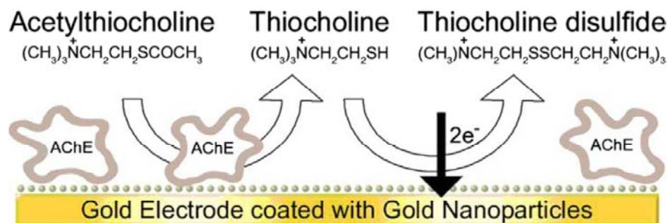
**Fig. (3).** Schematic diagram of the enzymatic reaction at the gold nanoparticle-coated AChE electrode. (*Electrochemistry Communications*, 2007, 9, 935).
