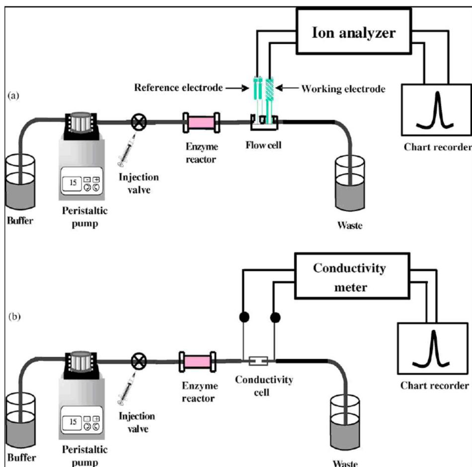
**Fig. (10).** Schematic diagram showing the flow-injection biosensor systems: (a) potentiometric; (b) conductimetric. (*Biosen. Bioelectronics*, 2005, 21, 445).
