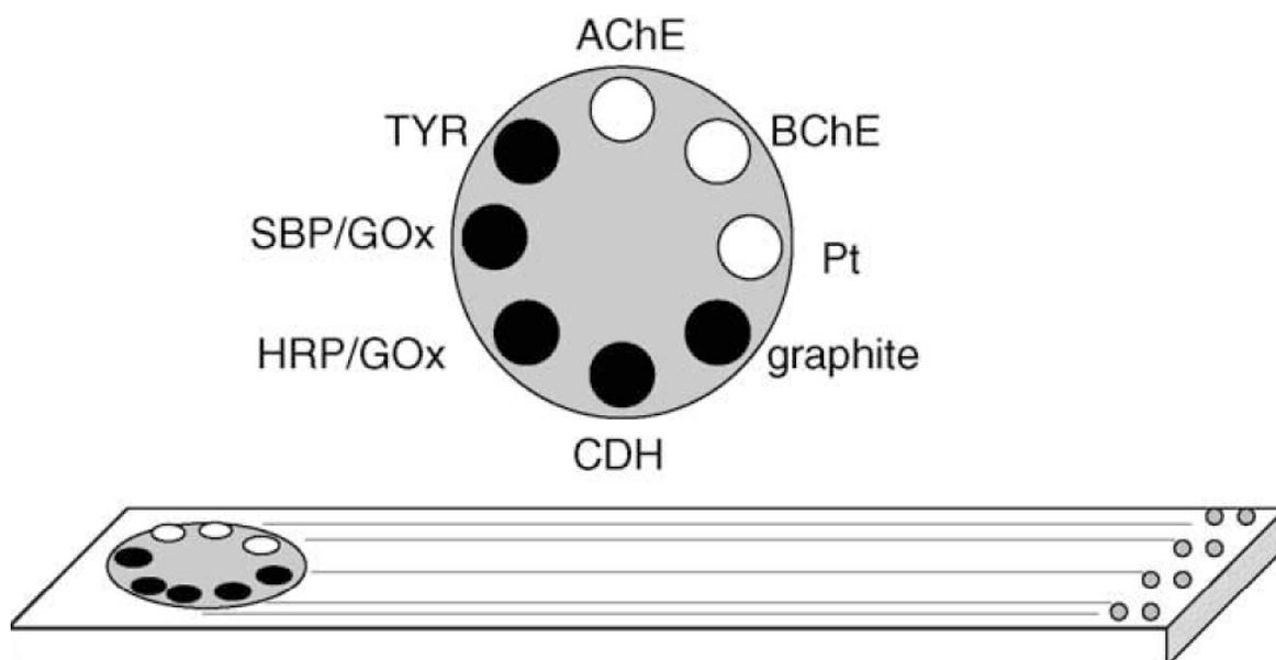
**Fig. (11).** The construction of the eight-electrode screen-printed array and the illustration of the final distribution of enzymes on the working electrodes, free Pt and graphite electrodes remained uncoated. (*Anal. Chim. Acta*, 2005, 528, 9).
