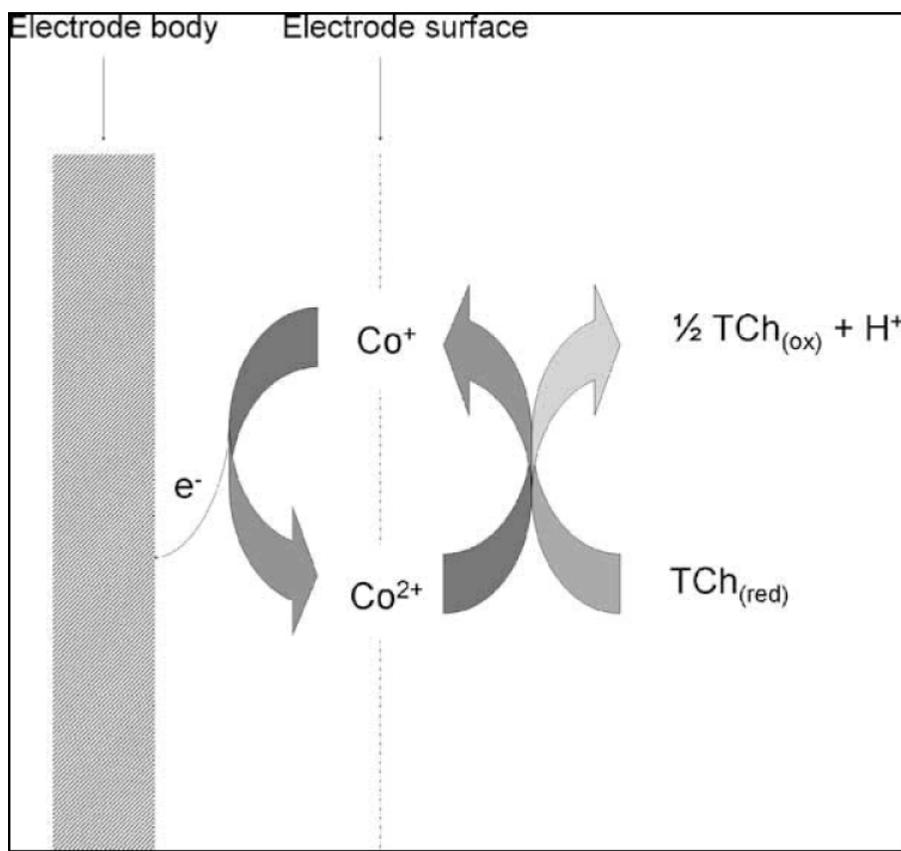
Fig. (8). Schematic representation of the Co-phthalocyanine mediated electrode surface. (*Biosens. Bioelectronics*, 2004, 20, 765).
