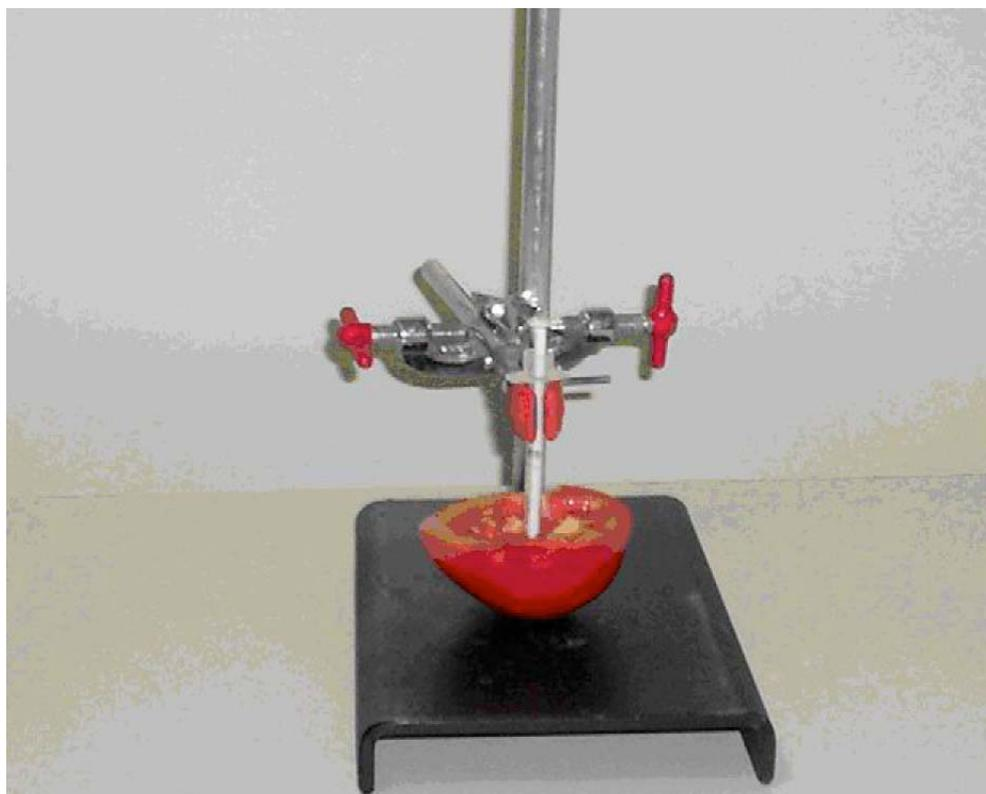
**Fig. (2).** Photograph of the experimental set-up for immersion of the biosensor in the Tomato "in natural", spiked with carbaryl. (*Sensors and Actuators B* 129, 2008, 40).
