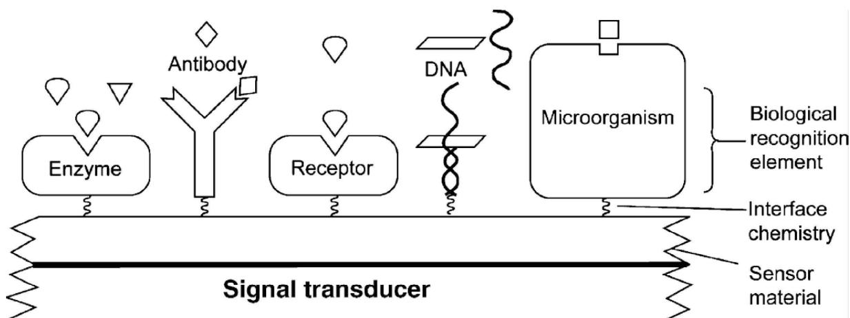
Fig. (1). Schematic representation of biosensors. (*Anal. Chim. Acta*, 2006, 568, 221).
