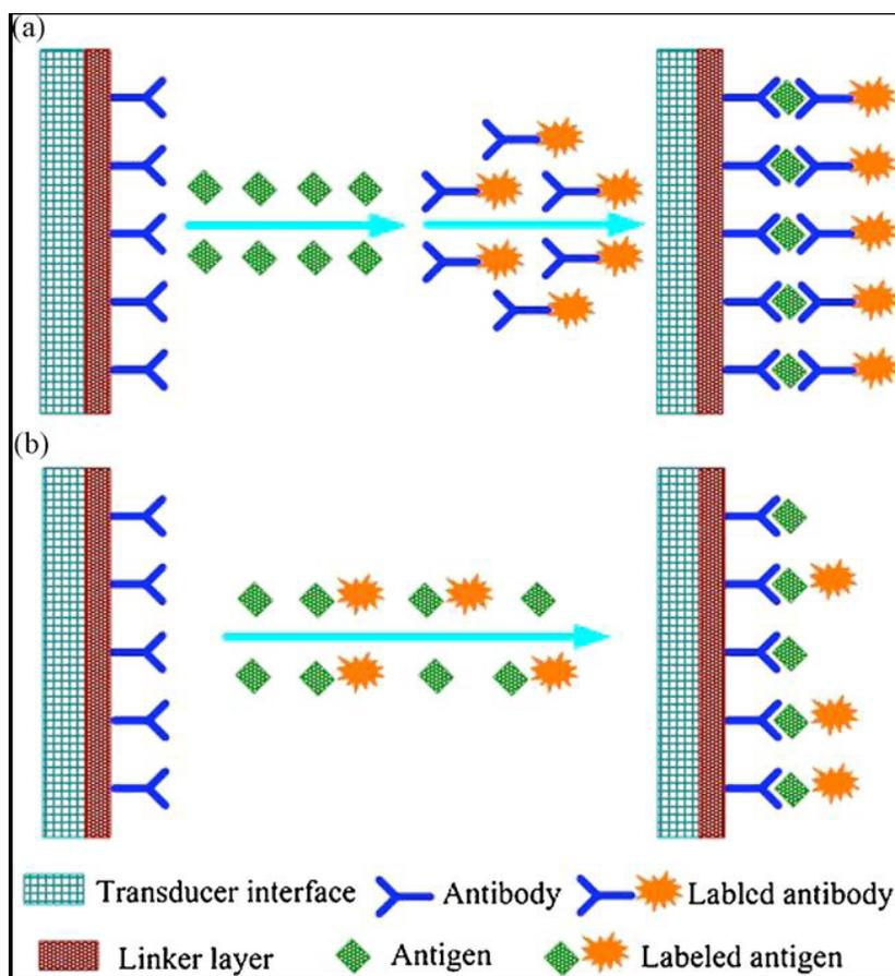
**Fig. (13).** Schematic of labeled immunosensors: (a) sandwich format and (b) competitive format. (*Biosens. Bioelectronics* 23(2008)1577).
