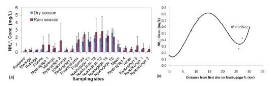
Fig. (8). NH<sub>4</sub>-N levels for (a) all the sampling sites and (b) sampling sites located on the Nyabugogo River for the monitored period.
