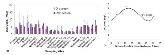
Fig. (6). Dissolved Oxygen levels for (a) all the sampling points and (b) sampling sites located on the Nyabugogo River for the monitored period.
