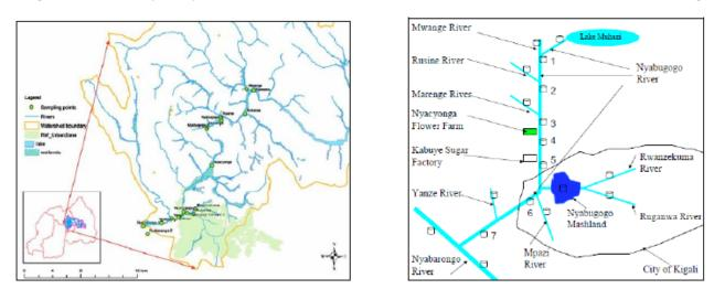
Fig. (2). Map of the Nyabugogo Catchment showing the location of sampling sites and a schematic chart of the monitoring network.
