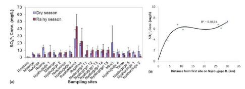
Fig. (11). Sulphate levels for (a) all the sampling sites and (b) sampling sites located on the Nyabugogo River for the monitored period.
