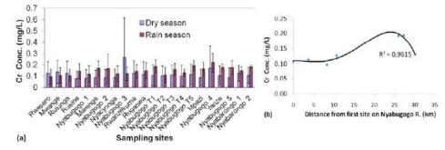
Fig. (18). Chromium levels for (a) all the sampling sites and (b) sampling located on the Nyabugogo River for the monitored period.
