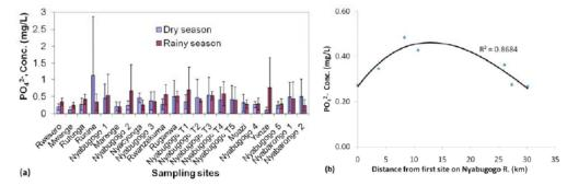
Fig. (12). Phosphate levels for (a) all the sampling sites and (b) sampling sites located on the Nyabugogo River for the monitored period.
