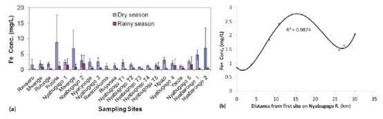
Fig. (15). Iron levels for (a) all the sampling sites and (b) sampling sites located on the Nyabugogo River for the monitored period.
