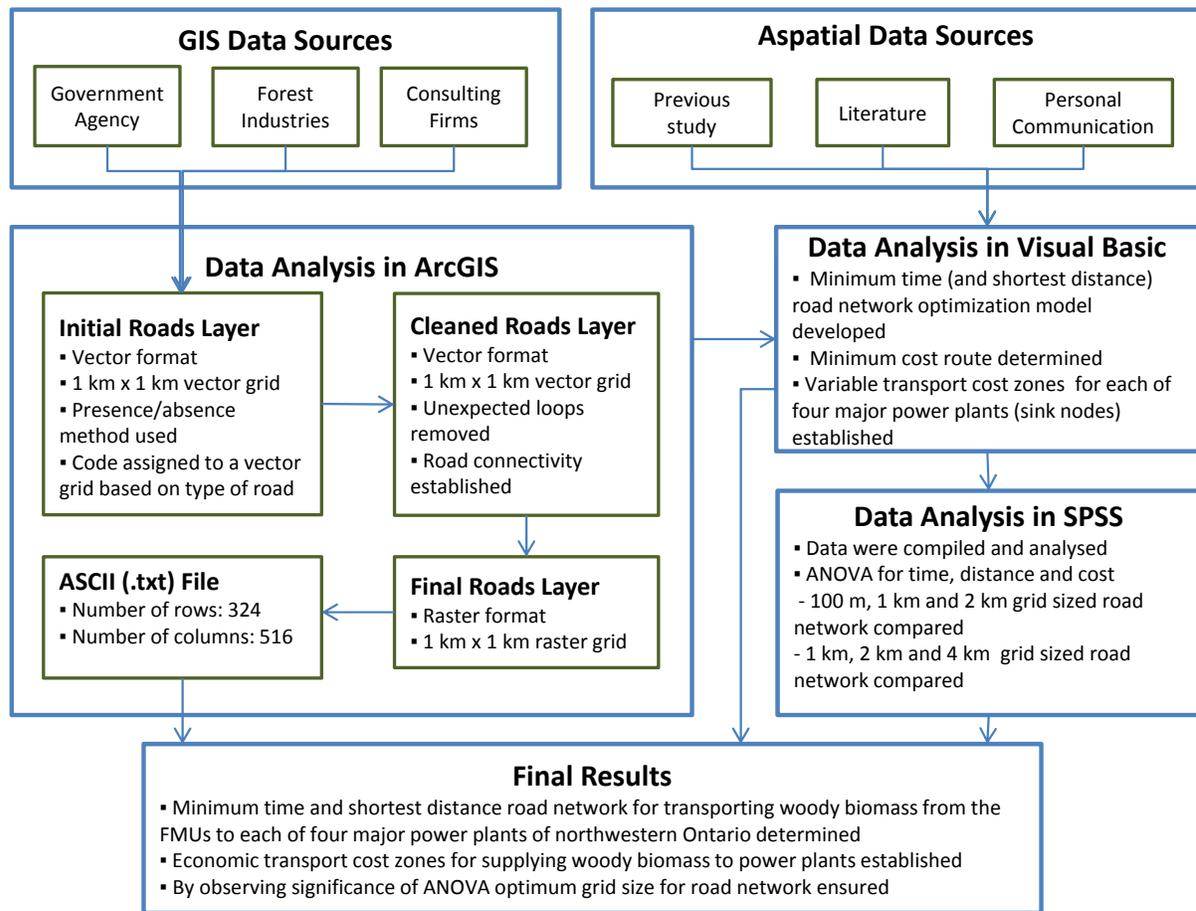
Fig. (2). Flow chart of GIS-based road network optimization model.
