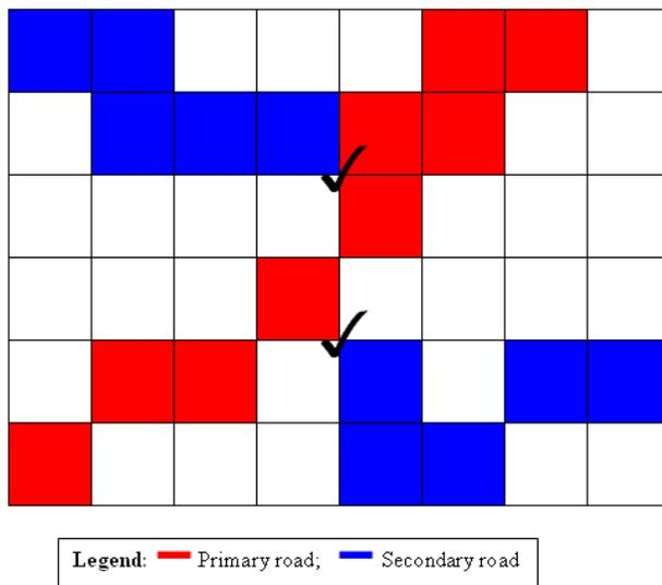
Fig. (4). Correct road intersection between two different classes of roads [25, 32].
