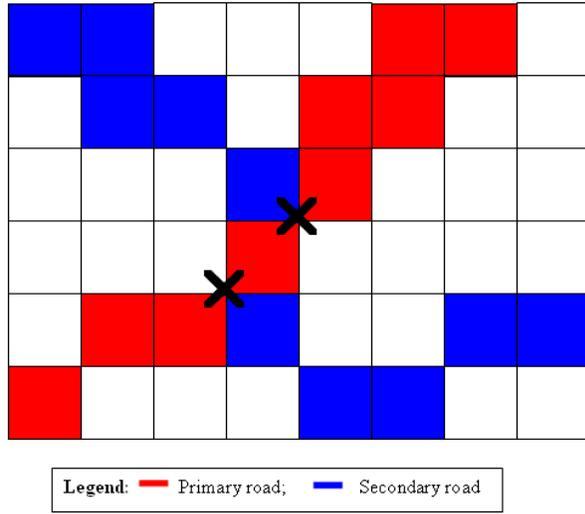
Fig. (3). Incorrect road intersection between two different classes of roads [25, 32].
