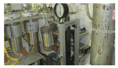
Fig. (9). Components of the homemade online subcritical adsorption-based device developed to allow effective CO<sub>2</sub> recycling.
