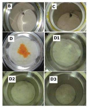
**Fig. (7).** Adsorbent materials used in the online subcritical adsorption-based device. B and C are Celite, and D is cotton. D1, D2 and D3 correspond to successive layers of cotton after removing the first layer seen in D.
