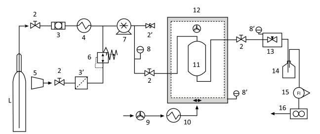
**Fig. (1).** SFE bench-scale unit. (1)  $CO_2$  cylinder, (2) blocking valve, (2') safety valve, (3) line filter, (3') air filter, (4) cooling bath, (5) compressor, (6) air pressure regulator, (7) air-driven fluid pump, (8) manometer, (8') temperature indicator, (9) blow motor, (10) blow motor resistor, (11) extraction column, (12) oven module, (13) micrometric valve with heating system, (14) collection flask, (15) flow meter, (16) flow totalizer.
