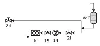
**Fig. (4).** Final step of the recycle system construction. Adsorption column (AdC) and other components as part of the recycle system of the pilot-scale unit. (2) blocking valve, (6) diaphragm flow meter, (AdC) adsorption column, (14) heat exchanger with electric resistance to heat the micrometering valve, (15) micrometering valve.
