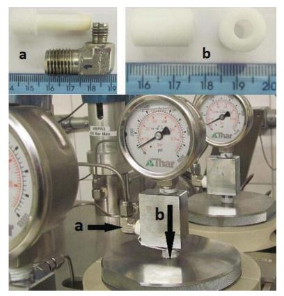
Fig. (8). Teflon bushings used to avoid the accumulation of extract in the SFE pilot-scale unit coupled with the developed online subcritical adsorption-based device.
