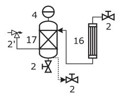
Fig. (3). Initial step of the recycle system construction. (2) blocking valve, (2') safety valve, (4) manometer, (16) shell and tube heat exchanger, (17) lung tank (LT).
