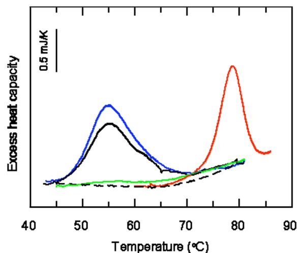
**Fig. (3).** DSC thermograms of cytochrome c – red line and its complexes with PVS – blue line and PSS – green line in 2 mM glycine buffer, pH 10.0. Black full line – 2. heating scan of cytochrome c – PVS complex; black dashed line - 2. heating scan of free cytochrome c.
